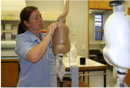
Carein Chan, technician, laminates a socket
